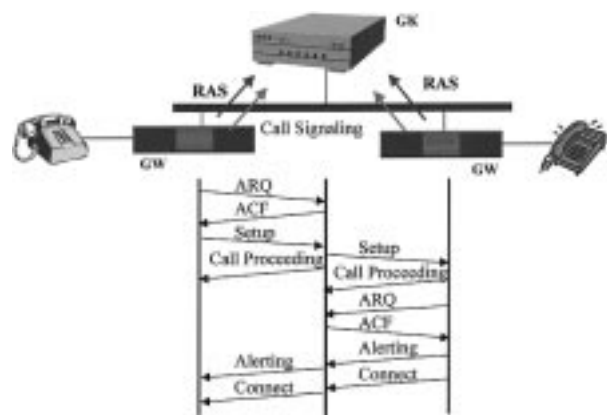
Fig. 12. Basic call setup with gatekeeper routed call signaling.
