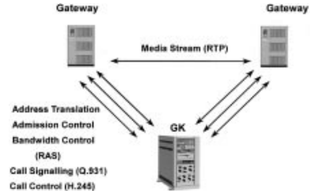
Fig. 10. Gatekeeper routed call signaling (Q.931/H.245).
